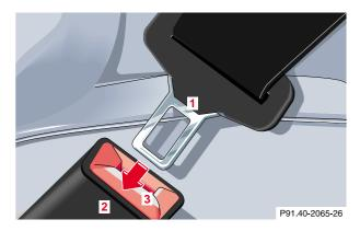
Push the release button (3) in the belt buckle (2). Allow the retractor to completely rewind the seat belt by guiding the latch plate (1).
